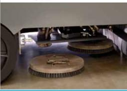
Widen the cleaning path from 40 in / 1020 mm up to 54 in / 1370 mm. Improve edgecleaning and maximize productivity with an optional side brush.
